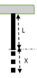
Let us consider the wire fitted to the roof of length 'L' and it has a cross-section area A is elongated to the new length by the action of a force.
