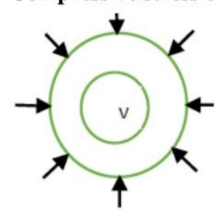
It is the uniform pressure (Force per unit area) acting normally all over the body. When the Deforming force is applied normally and uniformly to the entire surface of a body' it produces a volume strain (without changing its shape in case of solid bodies). The applied force per unit area gives normal stress or pressure. If F is the force applied uniformly and normally on a surface area.
