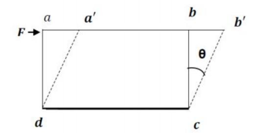
It is the force acting tangentially per unit area on the surface of a body. If a force is applied tangentially to a free portion of the body with another part being fixed, its layers slide one over the other; the body experiences a turning effect and changes its shape. This is called shearing and the angle through which the turning takes place is called shearing angle.
