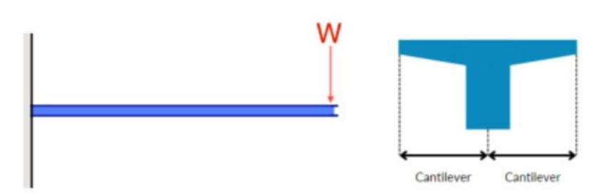
A good example of a cantilever beam is a balcony. A balcony is supported on one end only, the rest of the beam extends over open space; there is nothing supporting it on the other side. The cantilever beam is used in;
