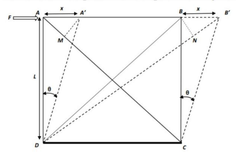
The diagonal element AC contracted to A'C similarly, the diagonal part BD is elongated to B'D
