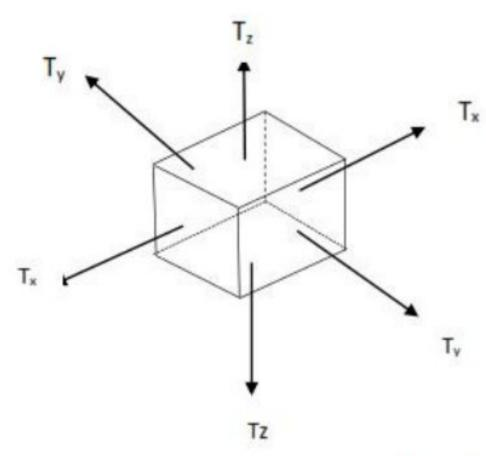
If the elongation stress produces the increase in the length along the x-axis then  $\alpha T_x$  is the strain.
