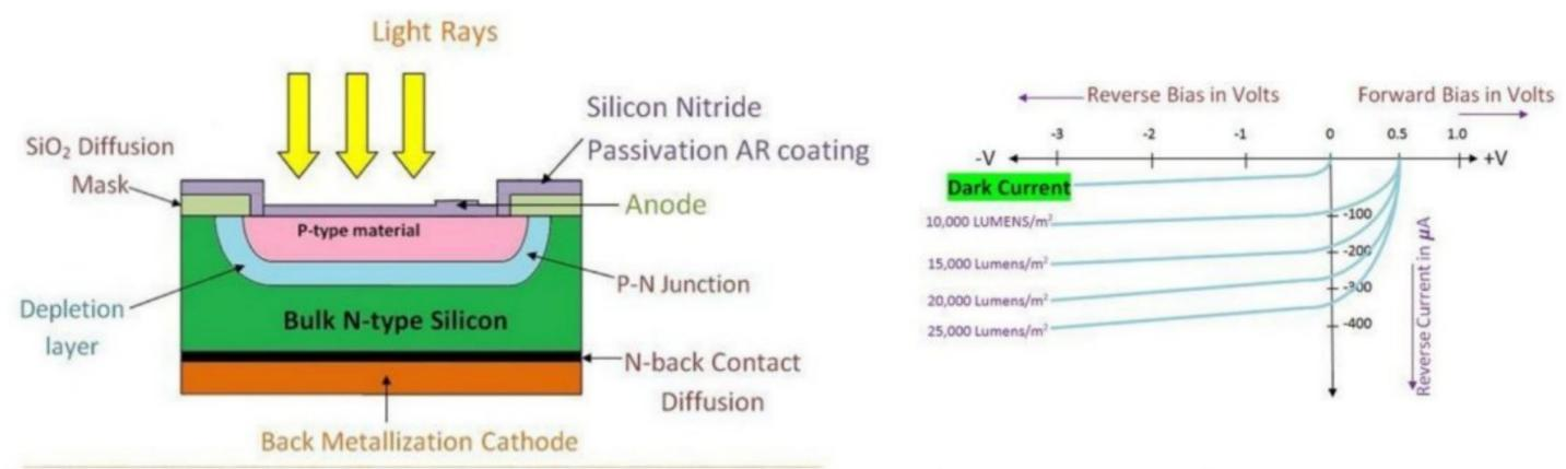
Construction: The photodiode is made up of two layers of P-type and Ntype semiconductor. In this, the P-type material is formed from diffusion of the lightly doped P-type substrate. The P+ diffusion layer is developed on N-type heavily doped epitaxial layer. The contacts are made up of metals to form two terminal cathode and anode.
