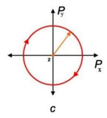
If the electric field having two orthogonal polarized components  $P_x$  and  $P_y$ of equal amplitudes but different in phase by 90°, then the wave is said to be circularly polarized.
