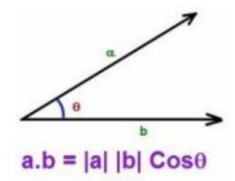
Example: Mechanical work is a dot product of force and displacement vectors, Power is the dot product of force and velocity, magnetic flux is the dot product of magnetic field and surface area.
