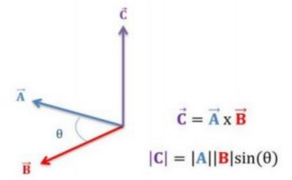
Example: Torque is the vector product of the force applied to a lever multiplied by its distance from the lever's rigid support.
