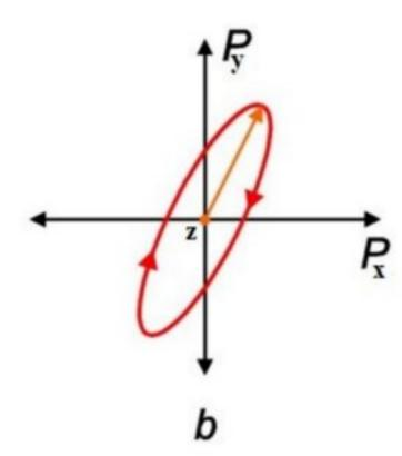
Elliptical polarization is a case where two waves of the same frequency, different phase, and different amplitude, combine into a single wave. The resulting vector P is the vector addition of the two field components  $P_x$  and  $P_y$ . The combined vector P appears to rotate in the pattern of an ellipse about the vector forming the direction of motion.
