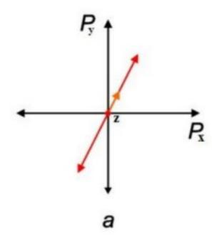
Linear polarization or plane polarization of electromagnetic waves is a confinement of the electric field vector or magnetic field vector to a given plane along the direction of propagation.
