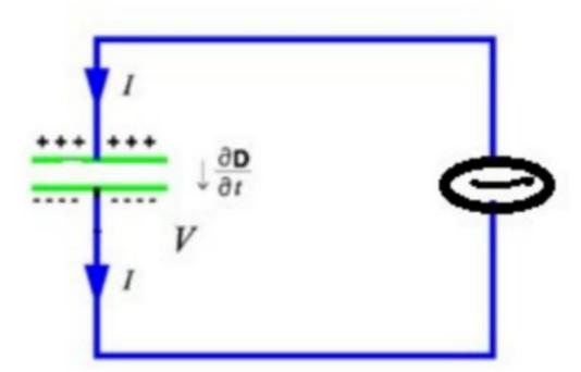
Consider a parallel plate capacitor connected across an A.C source. Let the area of each plate be 'A' and 'd' be their separation distance. Then the total potential for a parallel plate capacitor is given by,
