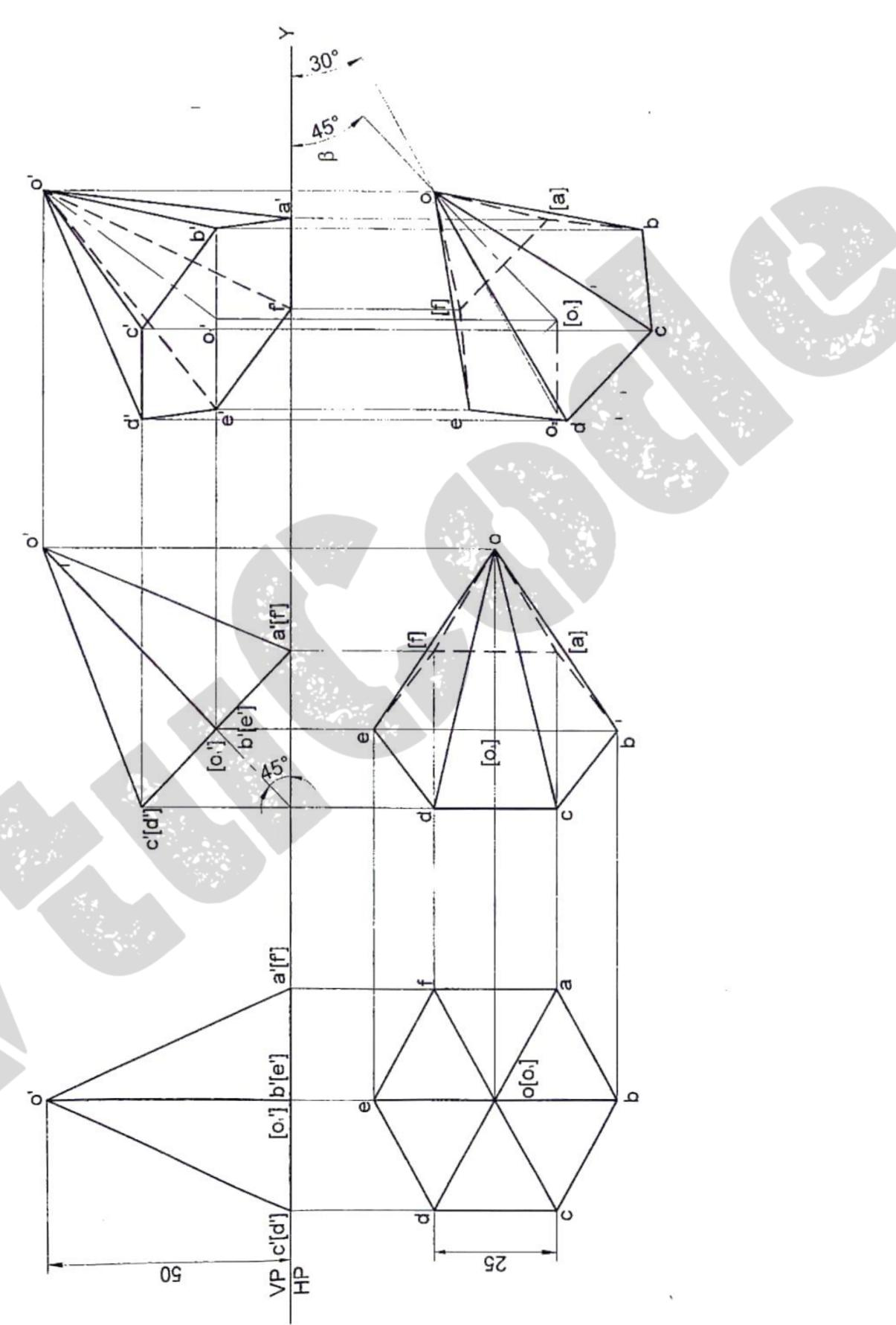
**Problem 26** A hexagonal pyramid 25 mm sides of base and 50 mm axis length rests on HP on one of its corners of the base such that the two base edges containing the corner on which it rests make equal inclinations with HP. Draw the projections of the pyramid when the axis of the pyramid is inclined to HP at 40° and appears to be inclined to VP at 45°.
